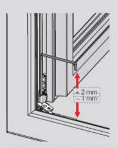
After the height adjustment, the load transfer device has to be readjusted (refer to page 51). Lateral adjustment
